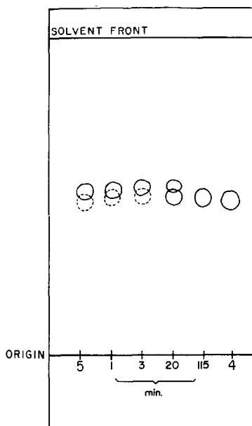
FIG. 2. Thin layer chromatographic analysis of isomerization of 5-androstene-3,17-dione by glycylglycine. The reaction mixture contained initially 0.04 M glycylglycine, pH 8.0, 0.184 mM 5-androstene-3,17-dione and 10% (v/v) methanol. At the indicated times during the reaction, 1.0 ml aliquots were extracted with chloroform and, after evaporation of the chloroform phase to dryness, spotted in ethanol solution onto the silica gel layer. The plate was developed with benzene-ethanol (9:1). In this solvent system 5-androstene-3,17-dione migrates just in front of 4-androstene-3,17-dione. The steroids were visualized as dark spots on a fluorescent background several hours after the developed plate was dried at room temperature. The lanes marked "5" and "4" contained 5-androstene-3,17-dione and 4-androstene-3,17-dione standards.
